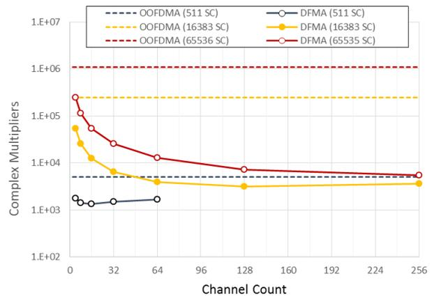
Figure 3. Complexity vs. Channel and Subcarrier counts
