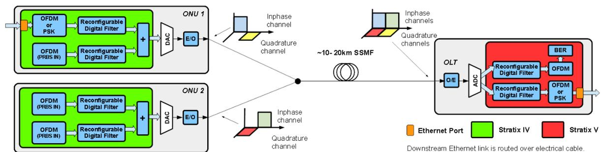
Figure 1. 4 channel DFMA PON Architecture
