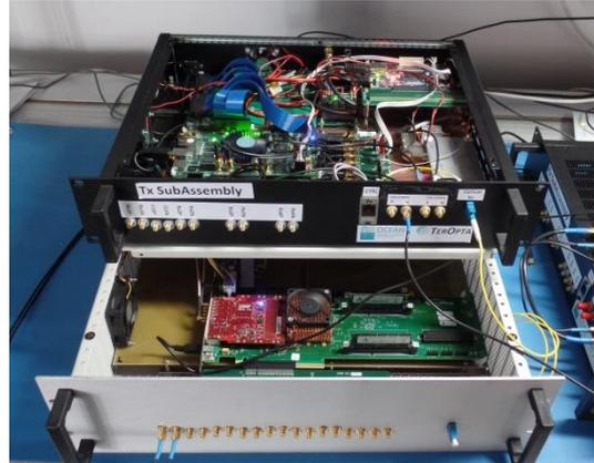
Figure 2. Demonstrator OLT and one ONU
